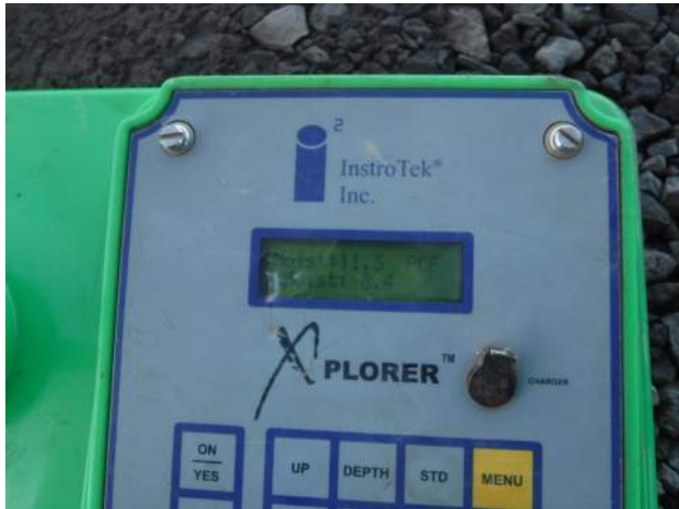
PCCP: PASHA maintenance blackout - Obtained 8.4 % moisture content
