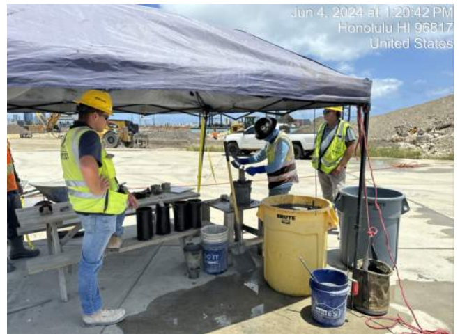
MPE performing slump loss testing for the CIDH mix
